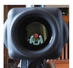
IMAGE - 3 Shows a LUCID HD7 with a properly adjusted reticle brightness as a sample of a proper reticle image.
