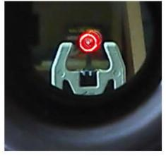
Shows a graphical representation of an Up and the the right directional reticle "Ghosting" due to Astigmatism.
